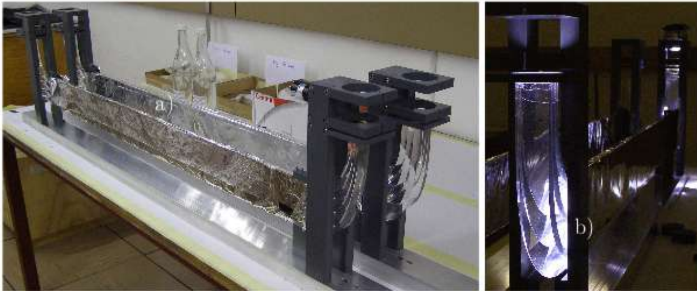
Figure 3.9: The K600 scintillator paddles. The material is insulated from external light sources by having the paddles wrapped in Mylar. The image on the right shows the light guides which couple the scintillators to their photomultiplier tubes [59].
