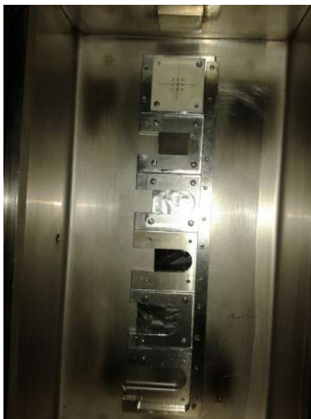
Figure 3.4: ^9\text{Be} and ^{26}\text{Mg} targets mounted on the K600 target ladder.
