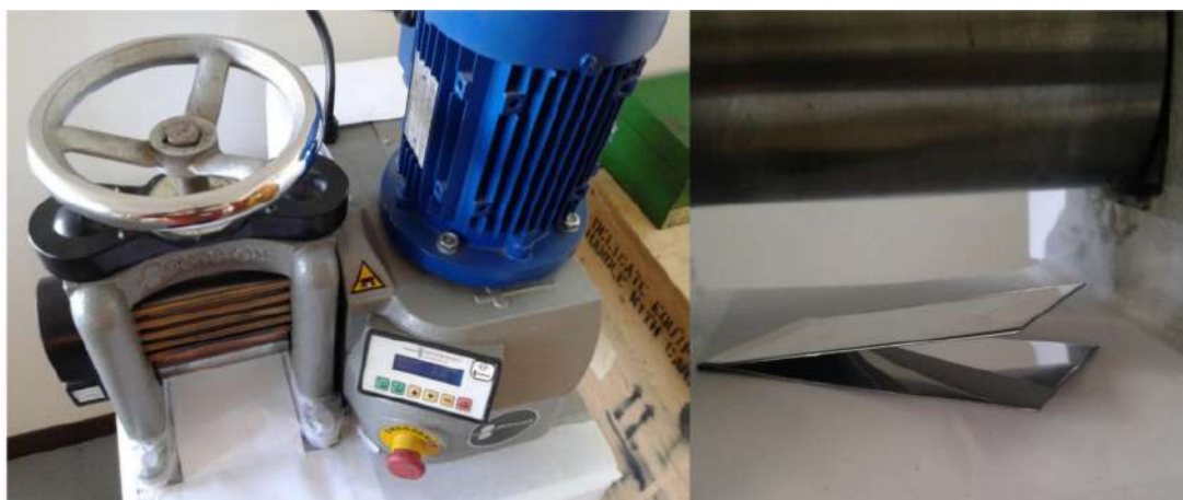
Figure 3.5: The mechanical rolling mill is shown on the left hand side and the stainless-steel pack on the right hand side.
