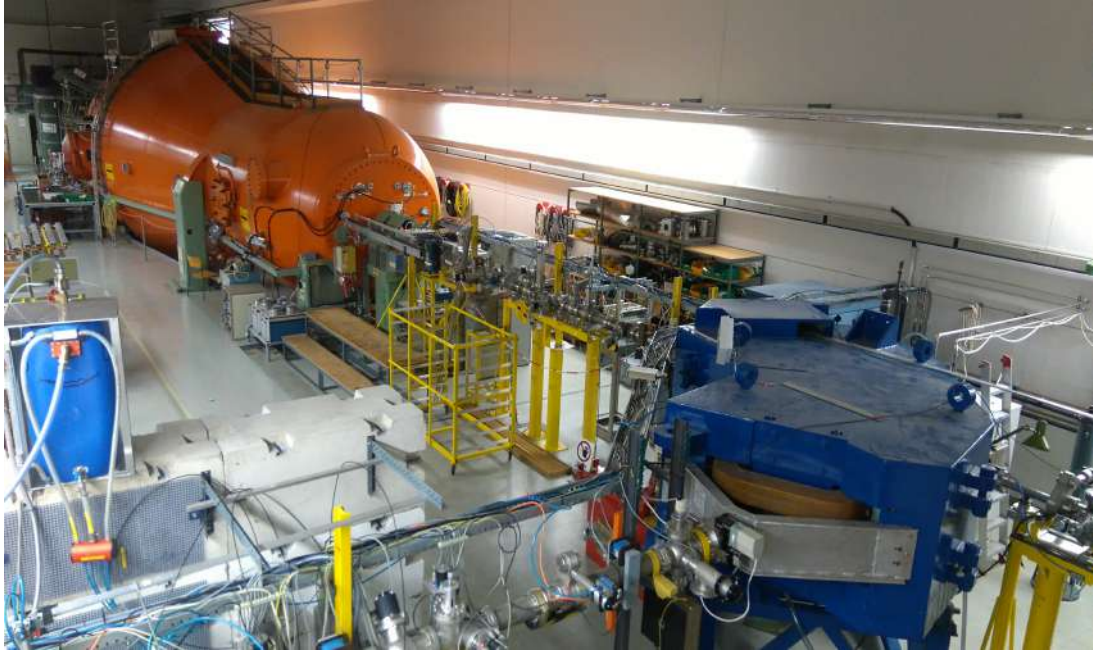
Figure 3.1: The tandem Van de Graff accelerator hall at MLL. The tandem is shown in orange and the analyzing magnet is painted blue.
