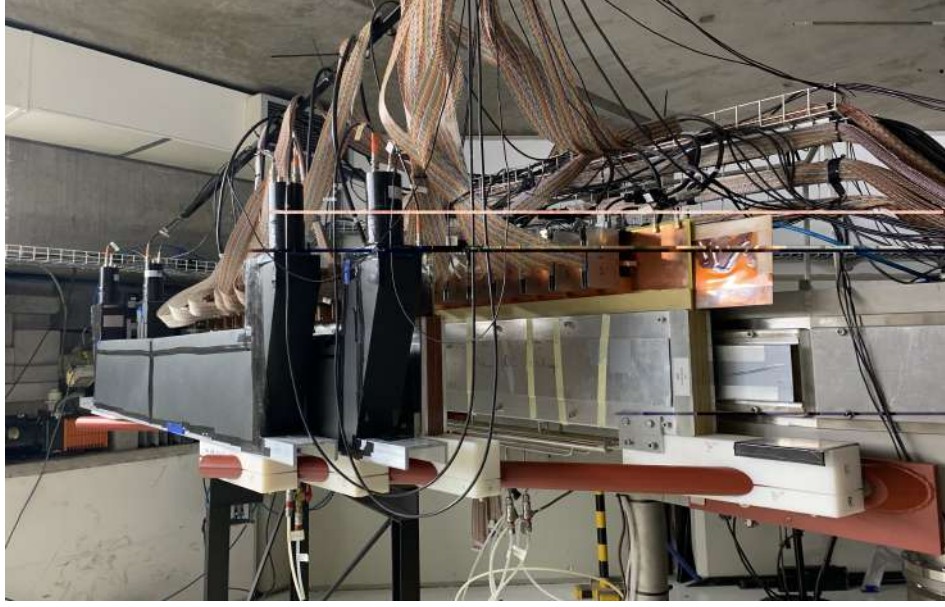
Figure 2.5: Position-sensitive drift chambers, with the plastic scintillator paddles at the focal plane of the K = 600 spectrometer. Figure taken from Ref. [28].
